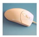
This has a rubber or metal ball on its underside that can roll in all directions. Mechanical sensors within the mouse detect the direction the ball is rolling and move the screen pointer accordingly.
